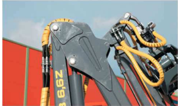
Make sure that the telescopic arm's locking hooks enter the holder on the lift arm
