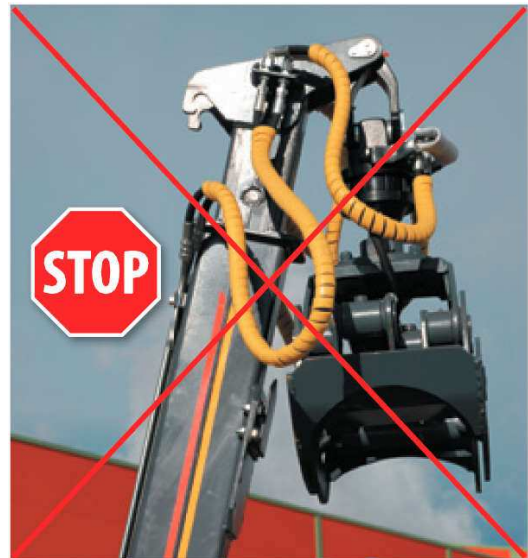
Make sure that the lock for the bucket/grapple engages with the lift arm
