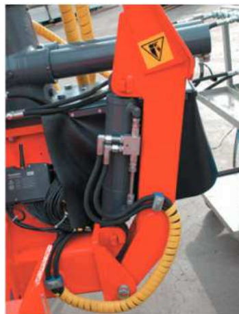
Counter balance valve for the support leg cylinders.
