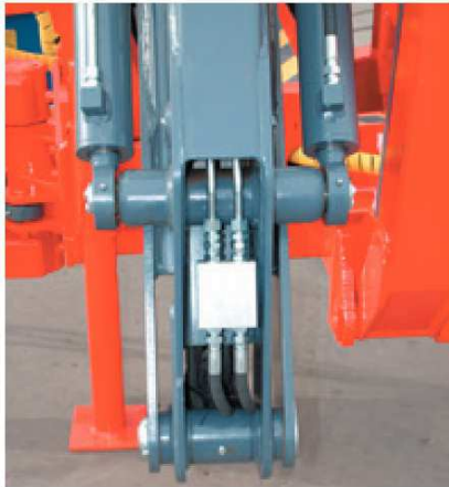
Counter balance valve for the telescopic cylinder.
