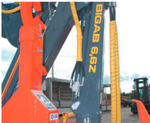
Counter balance valve for the lift cylinder.
