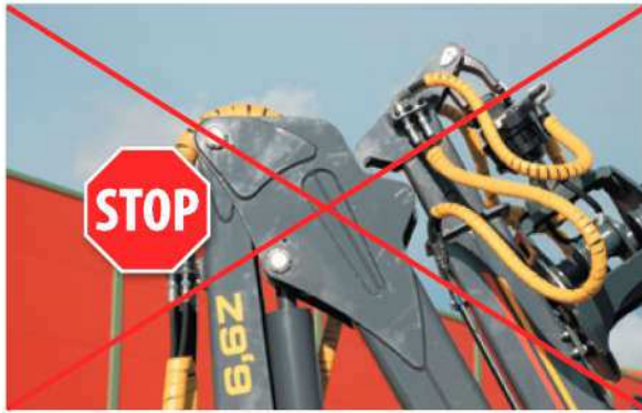
Make sure that the telescopic arm's locking hooks enter the holder on the lift arm
