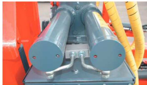
Counter balance valve for the turning cylinders.
