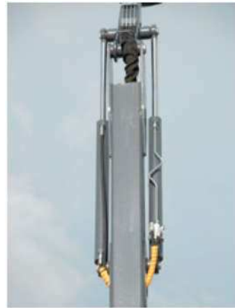
Counter balance valve for the outer cylinders.
