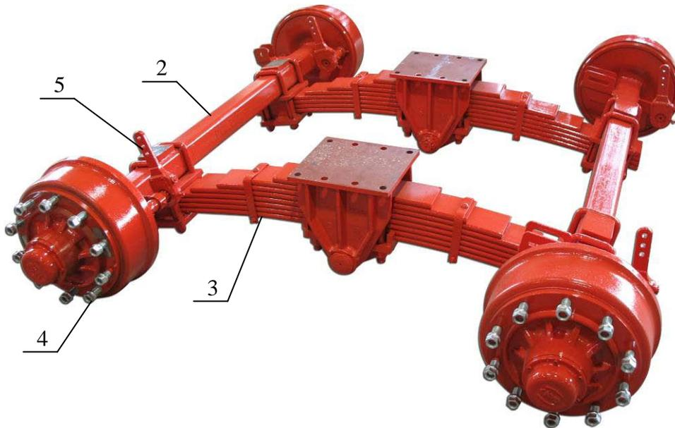
Figure 43. Boggie tandem suspendu
